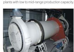
Rotary Drum Cooler side view.
